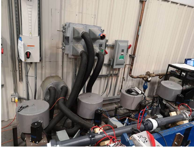
Figure 40. Connection of three PLAs to the exterior centrifugal fan; suction is applied from the top ducts while pressure is applied from the bottom
