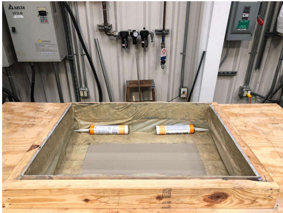
Figure 43. Latex sheet adhered over the vinyl siding and to the aluminum plates
